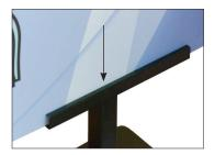
Set the graphic into groove of the Lower Graphic Fixture (5). Loosen screw on the Base Pole (2) and raise to the Top Pole (3) until the top fixture captures the rigid substrate. Once your graphic is secured in both grooves tighten the Base Pole Thumb Screw (7) by turning clockwise.
