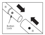
Connect (1) A-Left and (1) A-Right together to make a side of your triangle. Do this 6 times to construct the sides of your triangle. Set 3 aside for later use.
