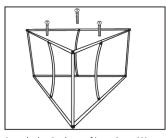
Attach the 2nd set of long bars (A) to the top of the curved side support bars (E) using the remaining shorts screws (D). Align the corners, but do
