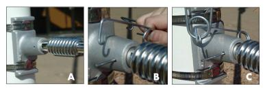
\*Pin should clip above casting
