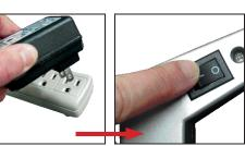
**Step 8** Plug lights (D) into power source and turn the switch on.
