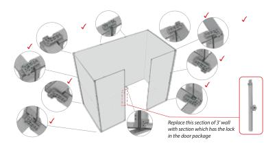
Correctly Setting up the 90° Corner Connectors (6) and wall placement is essential for proper enclosure setup.
