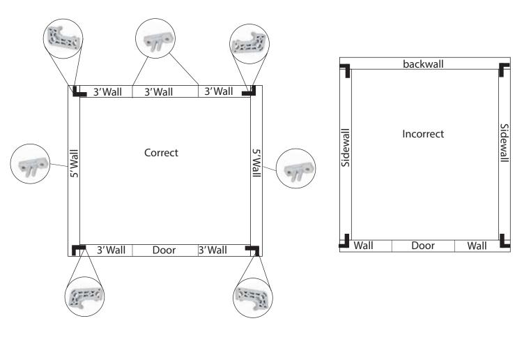
**Step 4**Attach 45° Top Corner Support Bars (11) to each top corner.
