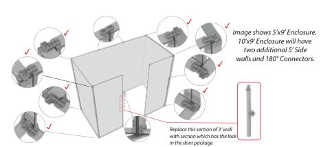
Correctly Setting up the 90° Corner Connectors (6) and wall placement is essential for proper enclosure setup.
