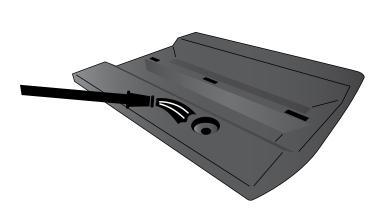
\*Base holds 2.3 gallons of water, weighing 24.5lbs when full
