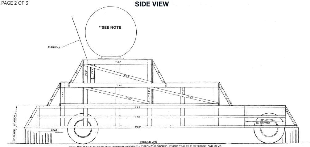
NOTE: THIS PLAN IS SCALED FOR A TRAILER PLATFORM 3' - 0" FROM THE GROUND. IF YOUR TRAILER IS DIFFERENT, ADD TO OR REDUCE APRON HEIGHT ACCORDINGLY. BEFORE STARTING CONSTRUCTION, CHECK ALL MEASUREMENTS AND MAKE ANY ALTERATIONS NECESSARY TO CONFORM TO THE TRAILER BEING USED.
